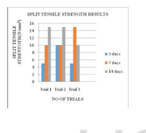
Pavement blocks Ratio of mix with quarry dust of 30%(P:F.A) = 1:3
