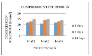
Pavement blocks Ratio of mix with quarry dust of 30% (P:F.A) = 1:3
